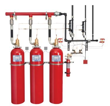
The SAPPHIRE PLUS system is most effective when used with an AUTOPULSE automatic detection and control system to release the clean agent rapidly. The detection system is used to either directly actuate a fire suppression system or to notify personnel that the system should be actuated by manual/pneumatic means.
